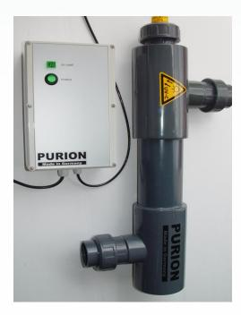
UV Plant PURION 2001 PVC is equipped with a PVC-U reactor. PURION 2001 PVC-U can be used to disinfect pool water up to a Volume of 30.000 I and for a transmission of at least 90% per cm. To ensure the required transmission a preliminary filter could be necessary. Other applications are fish ponds up to a volume of 30.000 l at continuous recirculation.
