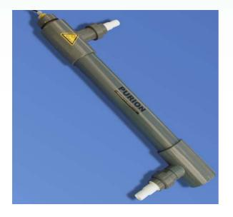
UV Plant PURION 2501 PVC is equipped with a PVC-U reactor. PURION 2501 PVC-U can be used to disinfect pool water up to a Volume of 50.000 I and for a transmission of at least 90% per cm. To ensure the required transmission a preliminary filter could be necessary. Other applications are fish ponds up to a volume of 50.000 I at continuous recirculation.
